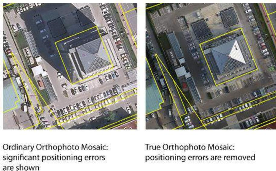
*Figure 2: Difference between ordinary and true orthophotographs. Note that ground objects are obscured in the ordinary orthophoto example. Photo courtesy Geavis.*
