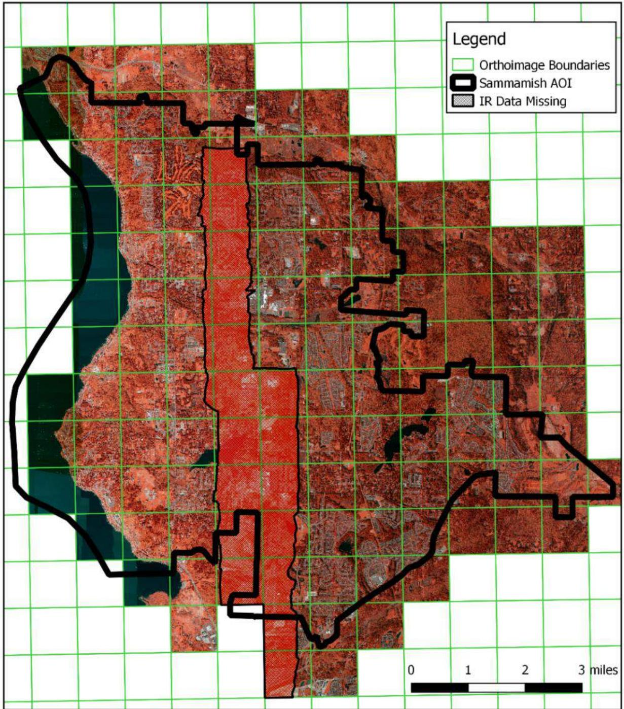
Figure 3: Map of the missing IR data in relation to the City of Sammamish area of interest boundary and orthoimagery tile boundaries. East, center (missing), and west sections of the city were analyzed separately. Orthoimagery shown in false color (IR band is red) to highlight missing data—IR values in this section are the maximum possible so the section appears red.
