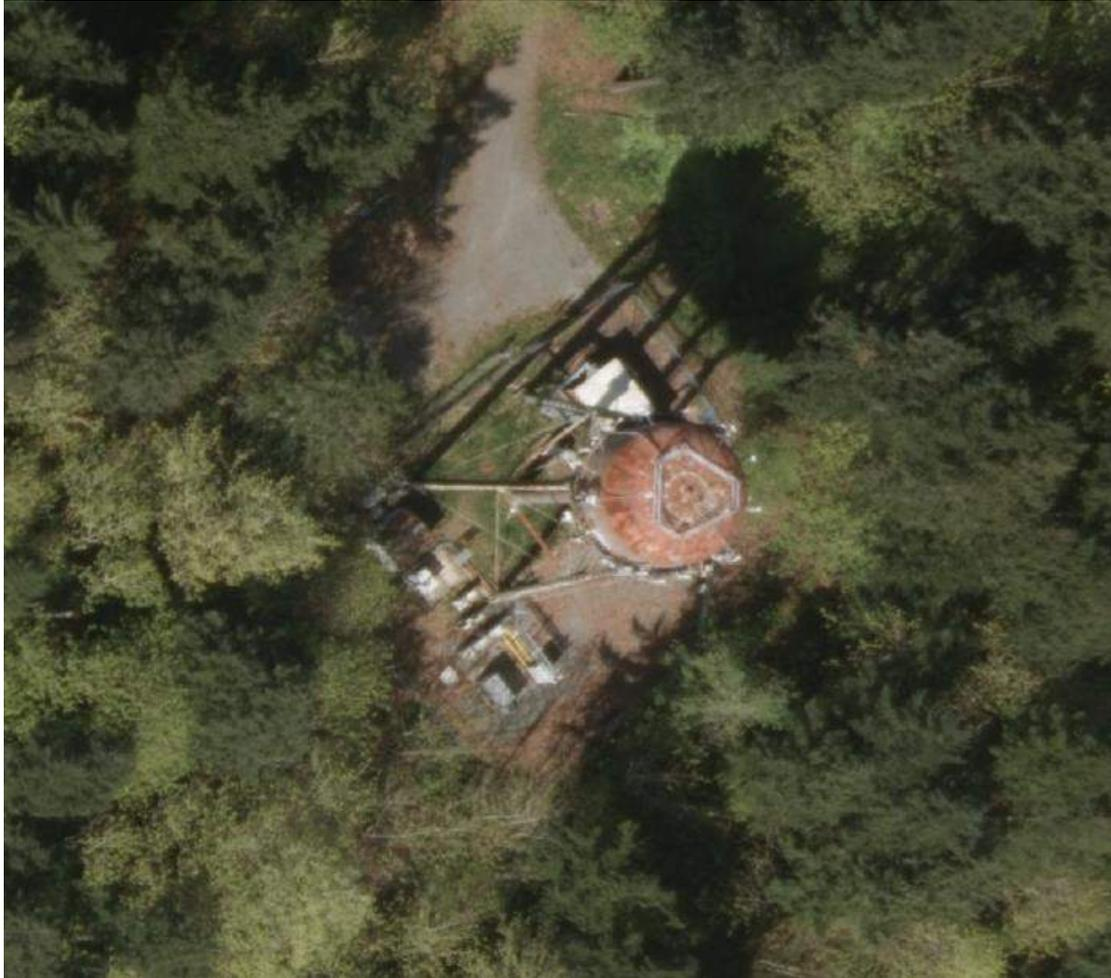
**Poor image stitching:** This image is poorly stitched together. This problem is caused by not overlapping aerial photography passes densely enough. Image artefacts like this create significant uncertainty in the model and increase error of the land cover classification.
