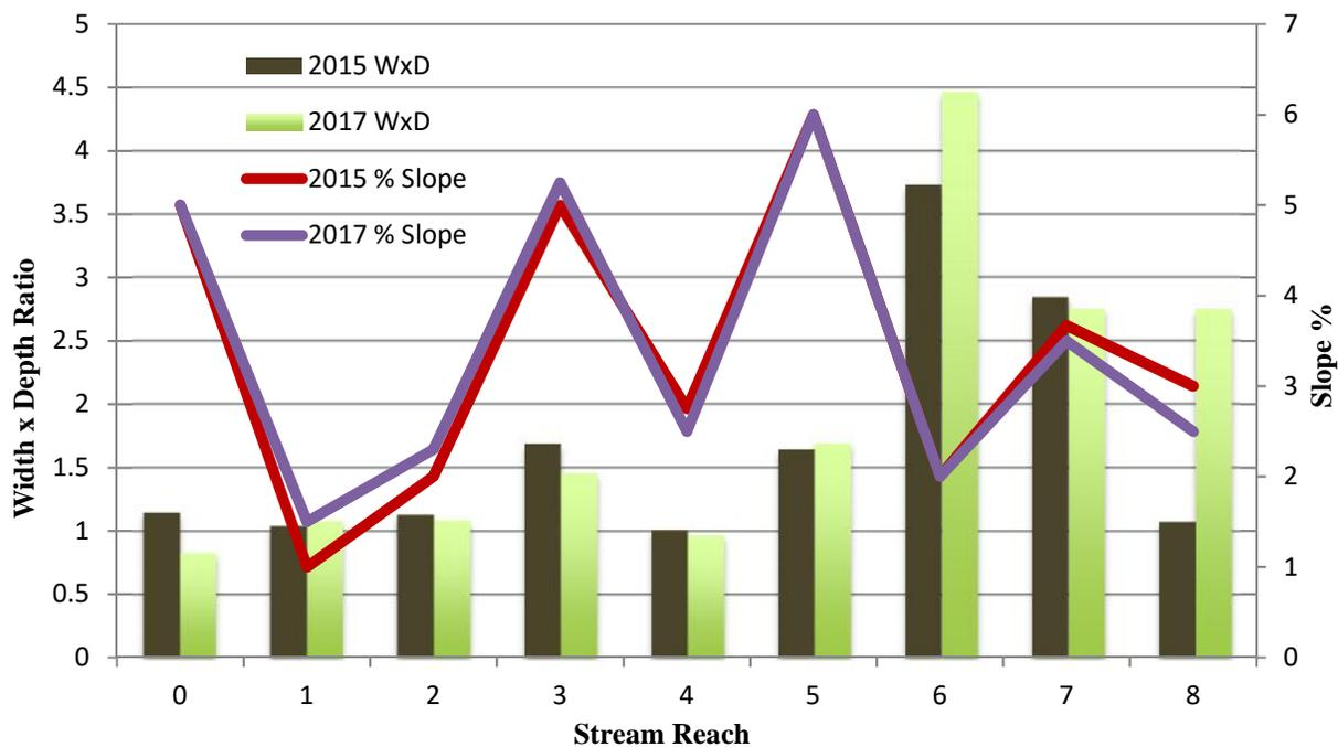
**Figure 3:** Width-to-Depth Ratio and Stream Channel Slope for Each Reach (2015 and 2017)
