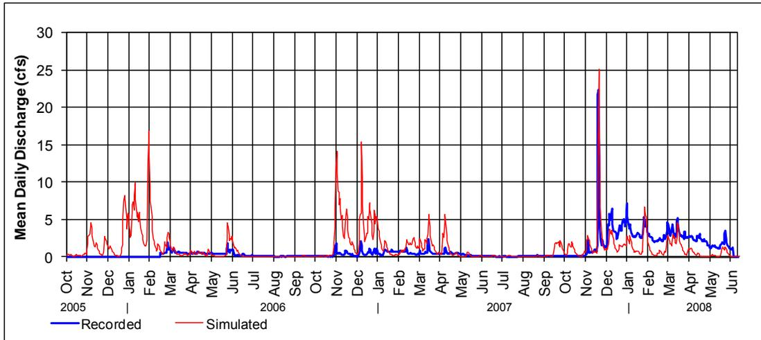
**Figure 8 – Comparison of Simulated and Recorded Flow at Mouth of Ebright Creek**
