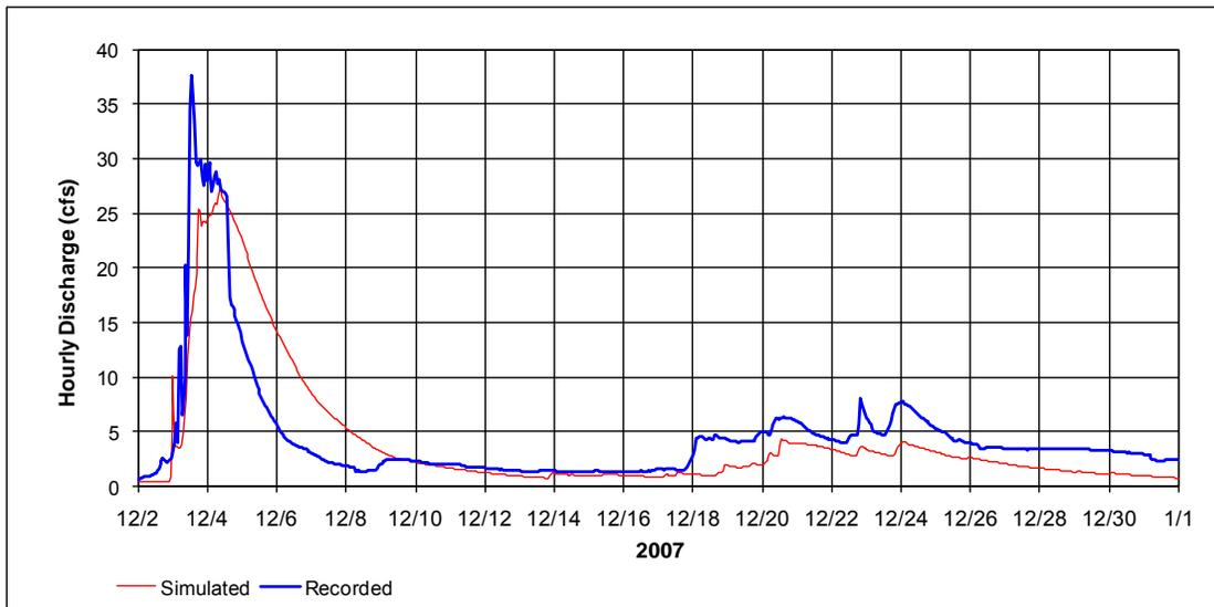
**Figure 9 – Comparison of Simulated and Recorded Flow at Mouth of Ebright Creek**
