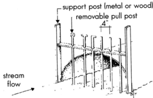
3. **Culvert Protector/Cleaner.** This alternative is similar to the Removable Pull Rod Grill, with the exception that the logging chain located at the top of the culvert is hooked to the bumper of a truck in order to lift the culvert cleaner out of the water to maintain and clean.
