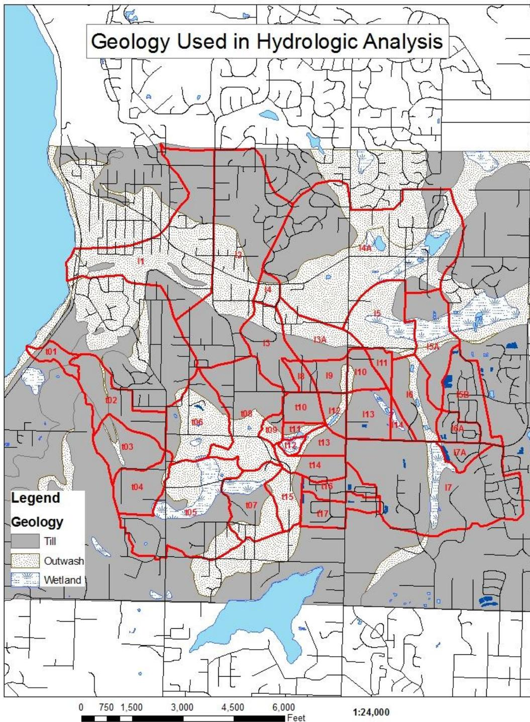
Figure 4 – Inglewood and Thompson Basins Geology as Defined for HSPF and MGSFlood Models
