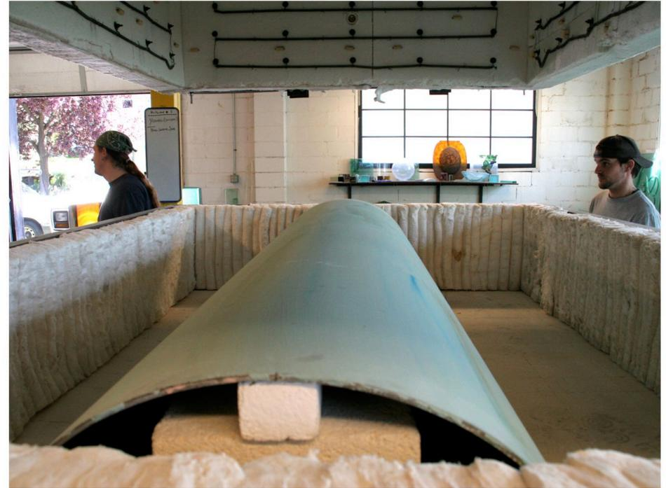
22 The glass slab is lifted into the kiln onto a rolled steel form for the "slump" firing that will give the glass the desired shape. The glass is brought up to temperature, slumped and annealed again to create the final elliptical work.
