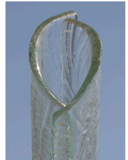
12 The original test firing for the glass scale model for "Confluence". The glass is originally fused flat and then slumped in a second firing into the desired curved shape.
