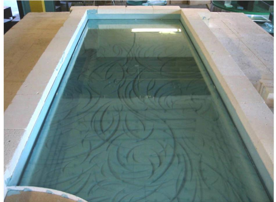
20 The mold is coated with a kiln wash release material and a dam is built to hold in the molten glass. 10 sheets of 1/4 inch plate glass are cut the shape of the mold and carefully stacked into the bed for firing.
