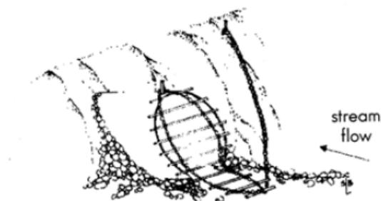
4. **Vertical Cylindrical Wire Mesh Beaver Guard.** This alternative protects the culvert inlet with a larger surface area than the previous two alternatives. The larger the wire mesh, the less maintenance needed to clear the debris.
