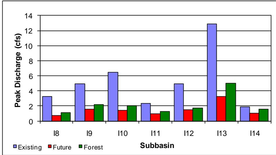
**Figure 13a – Town Center Subbasins in the Inglewood Basin, Comparison of 100-Year Flood Peak Discharge Existing, Future, and Forested Land Use**
