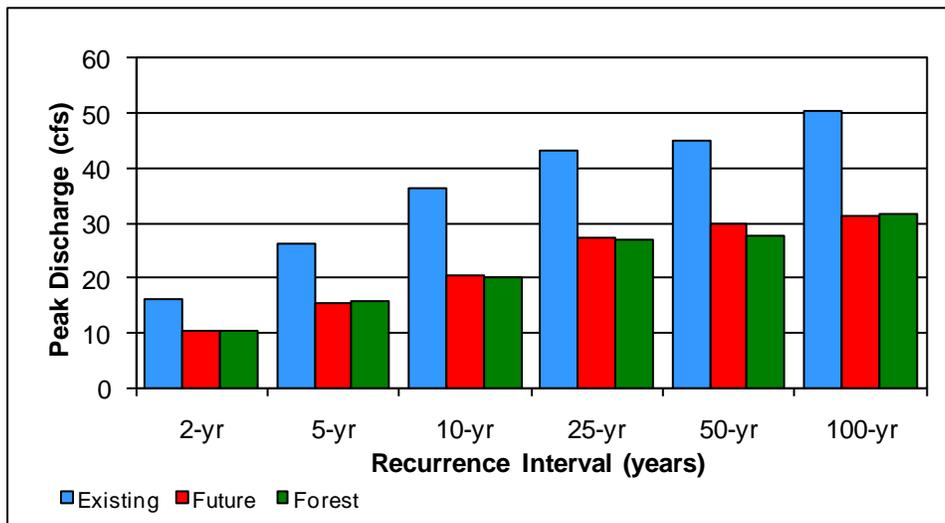
**Figure 12b – Comparison of Flood Peak Discharge at Mouth of Ebright Creek (Thompson Basin) Existing, Future, and Forested Land Use**
