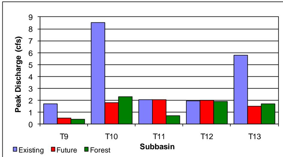
**Figure 13b – Town Center Subbasins in the Thompson Basin, Comparison of 100-Year Flood Peak Discharge Existing, Future, and Forested Land Use**
