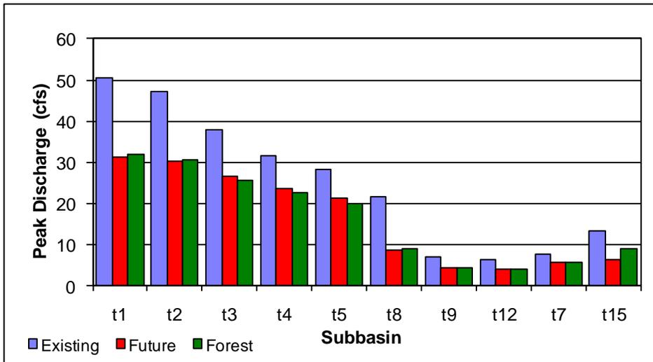
**Figure 12a – Ebright Creek, Comparison of 100-Year Flood Peak Discharge Existing, Future, and Forested Land Use**
