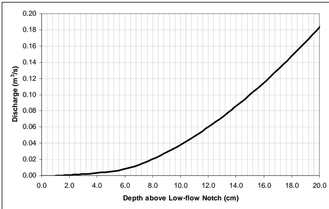
**Figure 16. Pine Lake Outlet Weir Rating Curve**
